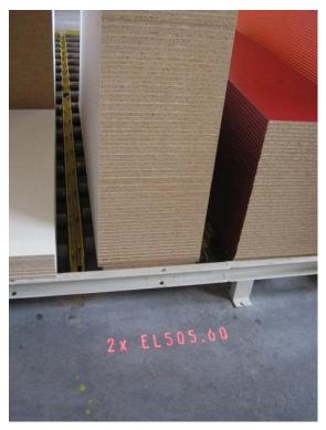
The laser projectors are mounted at the ceiling about 3.5 m high and display the amount to be picked and the article number of the parts required for the current production stage.
